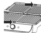
Open the Grill Toaster, locate the plate release buttons on front of the unit. Press firmly on button and the plate will pop up slightly from the base. Grasp the plate with two hands, slide it out from under the metal brackets, and lift it out of the base. Press on the other plate release button to remove the other cooking plate in the same manner.
